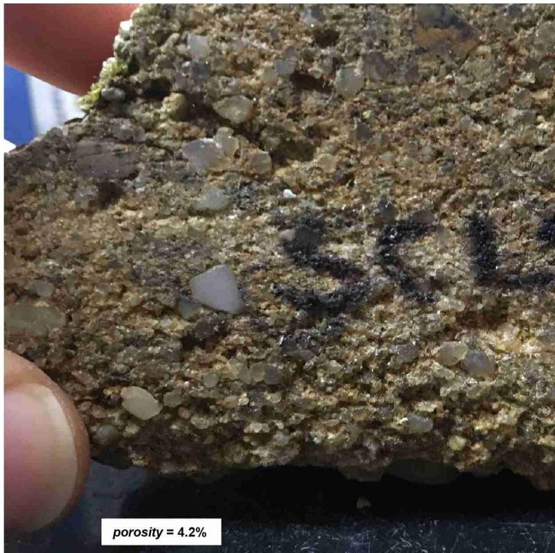
Figure 47. Photograph of hand sample L, Doswell Formation, Newfound Member. This hand sample is typical of conglomeratic, braided fluvial lithofacies association (LA B) sandstones.
